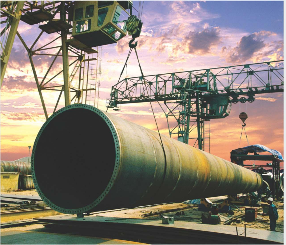
Chế tạo tháp Turbine gió xuất sang New Zealand. Fabrication of Wind towers for exportation to New Zealand.
